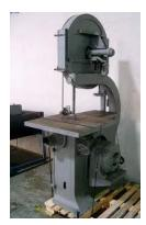
The 20" Band Saw has a thin vertical blade that allows cutting curves, re-sawing and large deep cuts on thick material. To avoid accidents the following operational safety rules must be observed by everyone working on the GWG 20" Band Saw. Failure to be certified or to follow the safety rules will result in loss of shop privileges.
